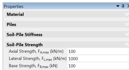
Figure 24.4: Parameters for Pile Rows (Soil-Pile Strength).
