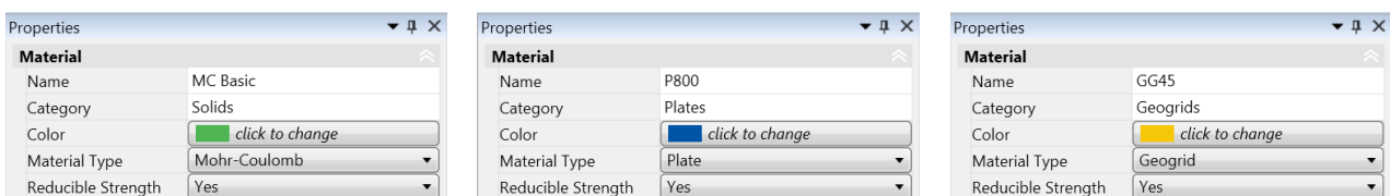
Figure 5.1: Properties of three materials belonging to the Solids (left), Beams (center) and Geogrids (right) categories respectively.
